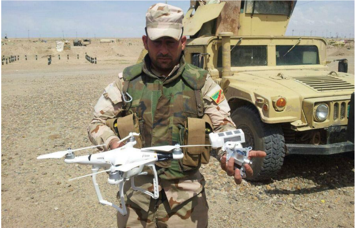
Caption #2: An Iraqi Security Force officer holding the ISIS' weaponized commercial quadcopters they deploy to the defense force. However, these drones are currently still battery operated and small, which means they could be taken down by the forces using signal jammers.
